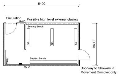
Floor Area shown 22.05 sq.m ALTERNATIVE WHEN SEPARATE ACCESS CHANGEROOM NOT PROVIDED
